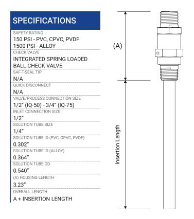
The IQ series non-retractable is well suited to small scale applications or those where the main can easily be depressurized to allow for servicing. The integrated check valve provides convenient isolation from the process pressure. Its size and availability in PVDF, C276, and Alloy20 make it ideal for sulfuric acid applications.
